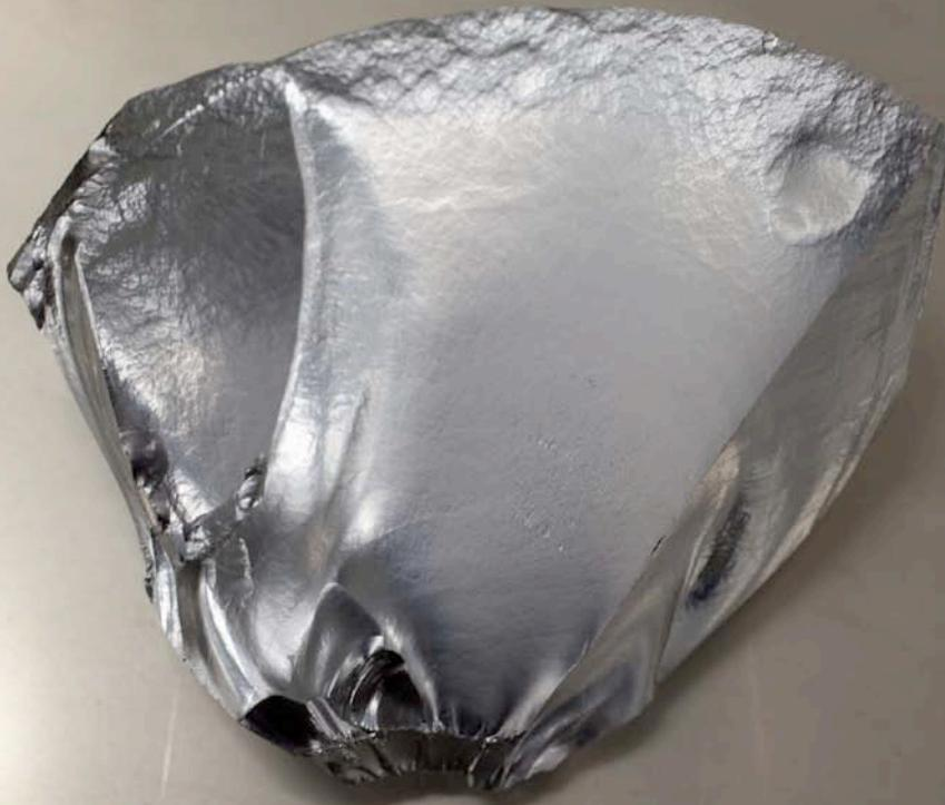
Schmid Silicon Technology's polysilicon has a high purity level that corresponds to 11N, 99,999.999.999% and can be applied in a broad range of industries.
