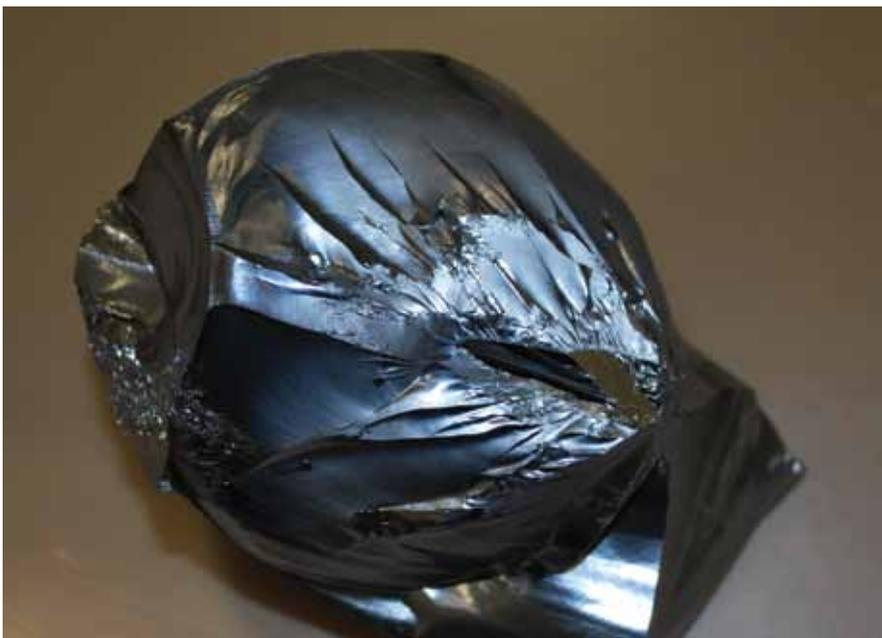
Monosilane-based, electronic grade polysilicon
